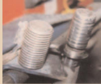
*The larger head on the left places shallower cuts than the narrower head on the right.*
